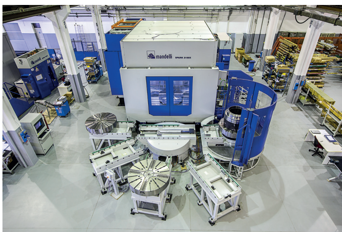
The new Mandelli machine SPARK 2100 A/T represents an extension of the turning-milling multitasking line
