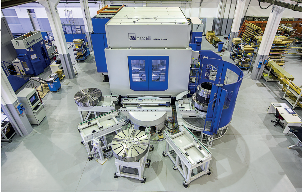
Spark can be equipped with tool magazines from 100 to 500 pockets. The unmanned production is possible thanks to roto-translating pallet systems and to several machining centers connected in FMS
