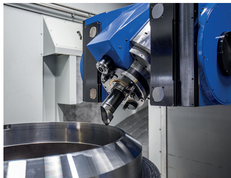
Spark can be equipped with tool magazines from 100 to 500 pockets. The unmanned production is possible thanks to roto-translating pallet systems and to several machining centers connected in FMS
