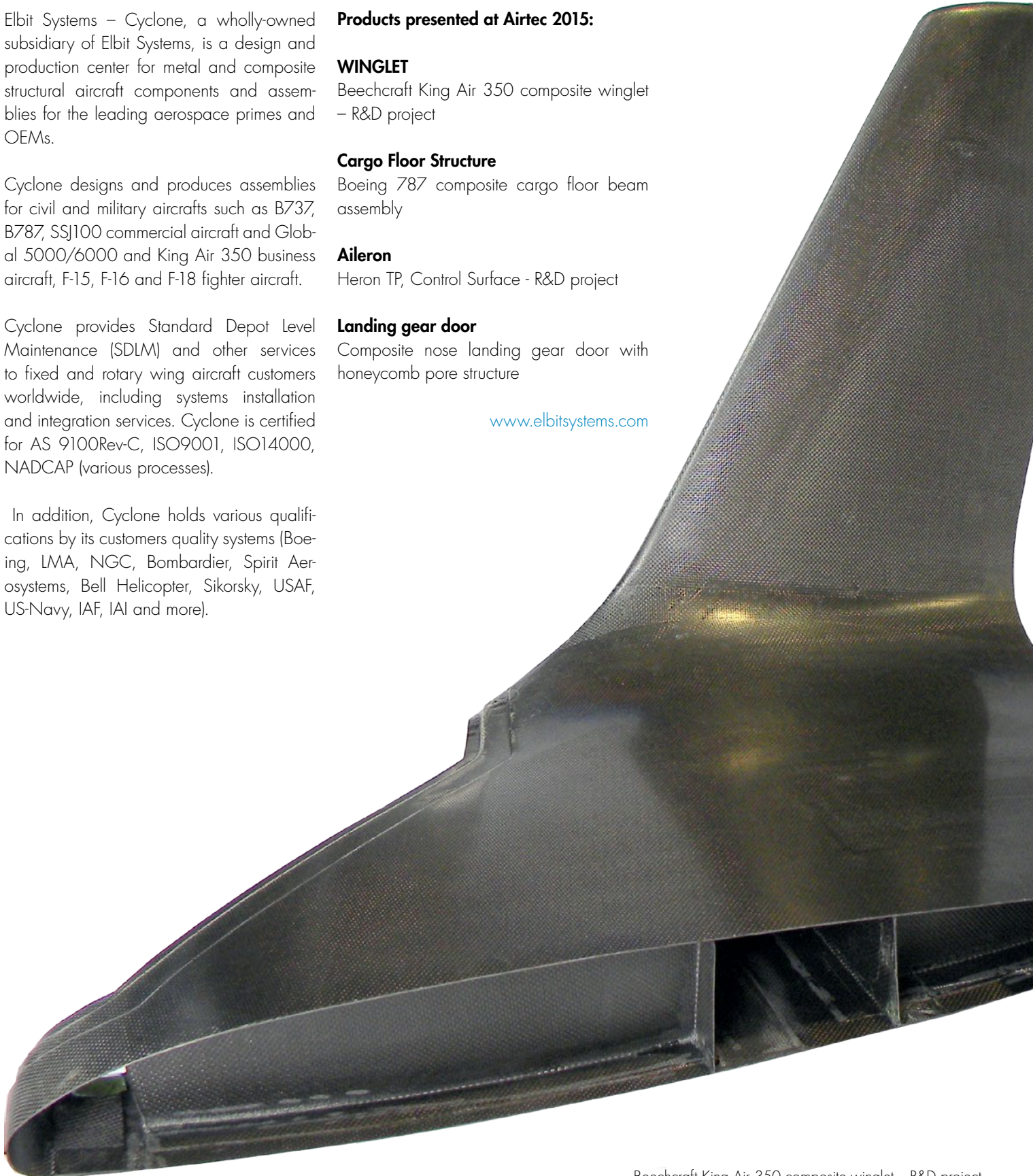
Beechcraft King Air 350 composite winglet – R&D project
