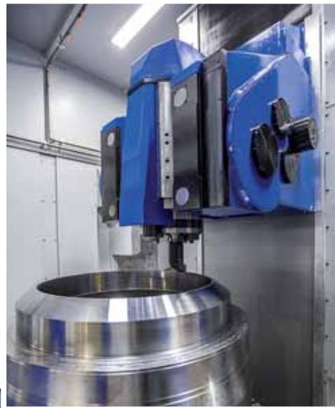
The turning head and turning table on Spark 2100 Milling /Turning.
