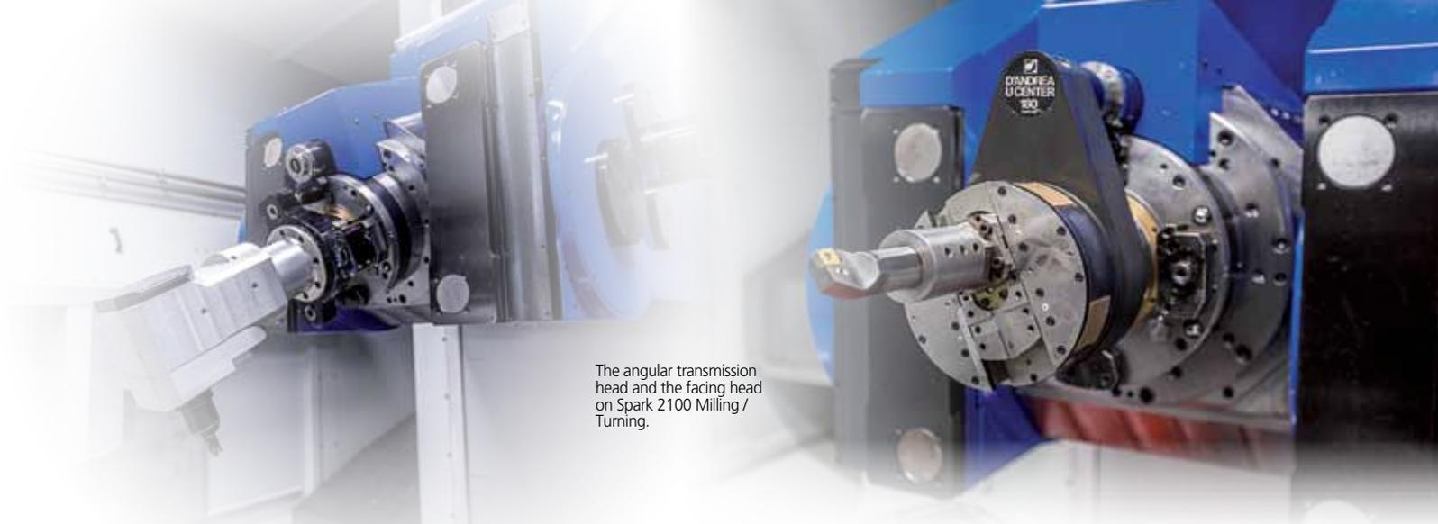
The angular transmission head and the facing head on Spark 2100 Milling / Turning.
