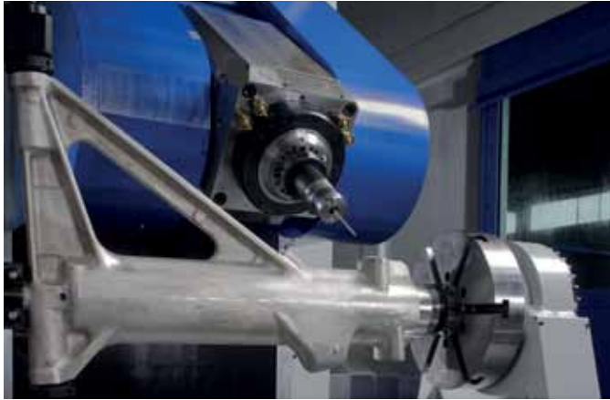
Left: machining of a landing gear section on Spark 2100X Right: a Mandelli application at SABCA
