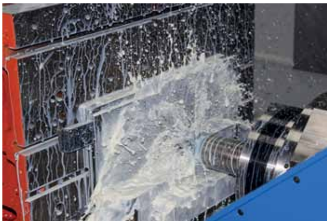
Mandelli's Spark while machining with coolant through spindle
