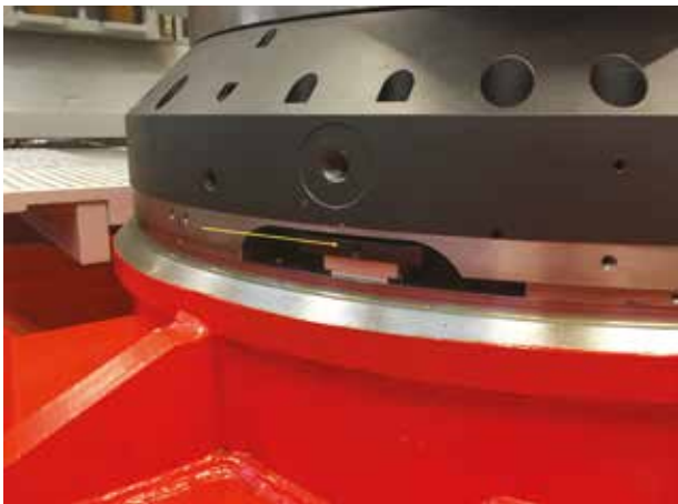
The turning table with the "bad balance sensor"
