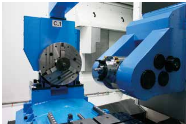
The holes on the shaft are interpolated between the spindle axis and the dividing head axis, both equipped with linear motor
