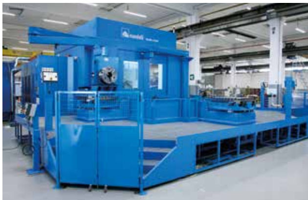
Rigidity and stability are important factors on HMCs like Spark as it machines extremely tough materials
