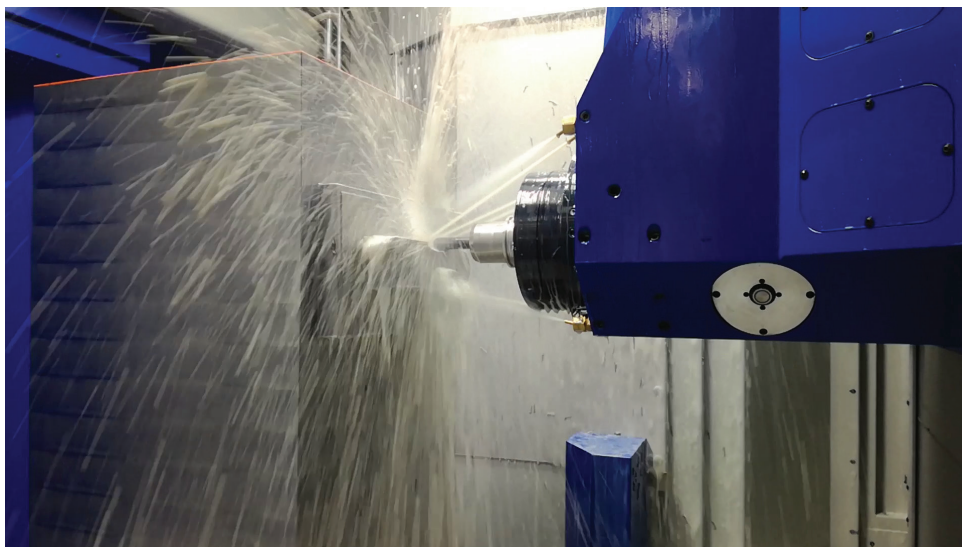
The high coolant flow is strategic to machine titanium
