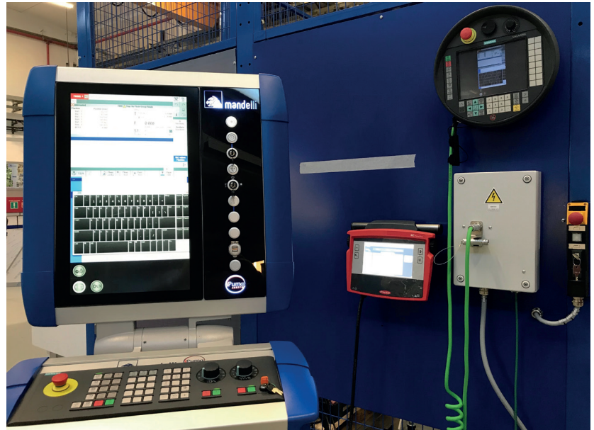
Left : Sp@rk-4.0-I.E.S. is a prototype of an automated cell that integrates a Spark 5-Axis HMC and an additive manufacturing robot station
