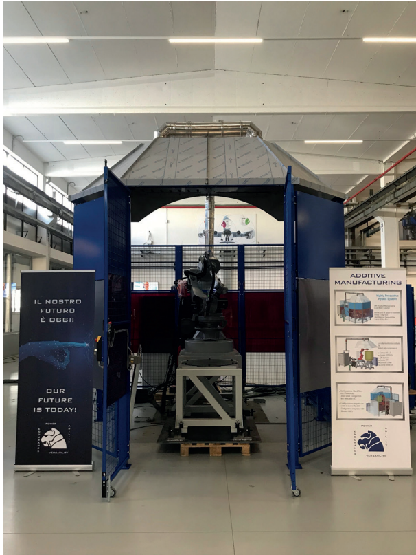
Left : Sp@rk-4.0-I.E.S. is a prototype of an automated cell that integrates a Spark 5-Axis HMC and an additive manufacturing robot station
