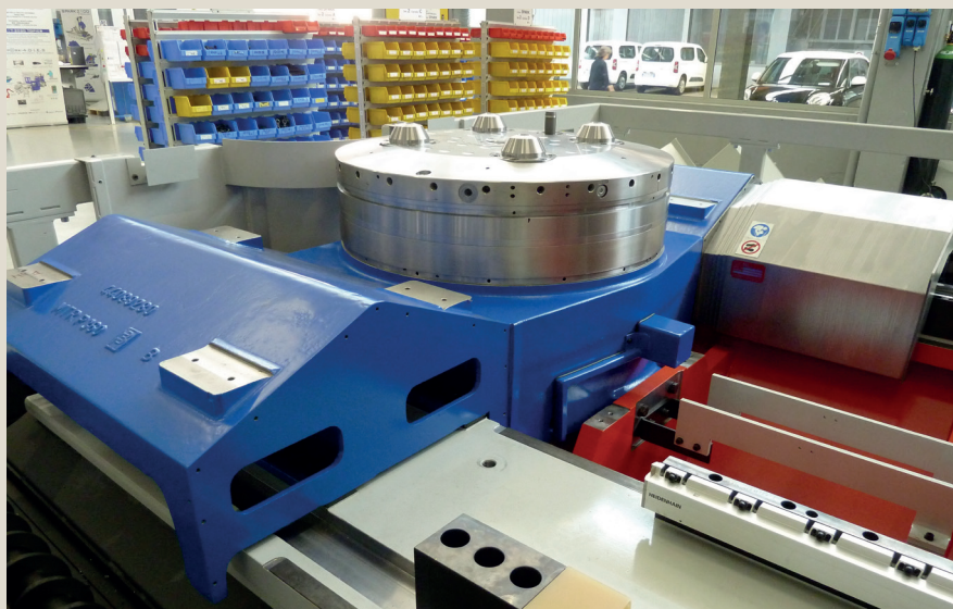
The rotary table is housed into the base to guarantee the highest turning performance
