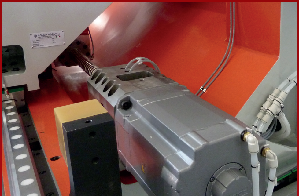
The possibility to have a double worm-screw on all the linear axes ensures a perfect balance of the work forces
